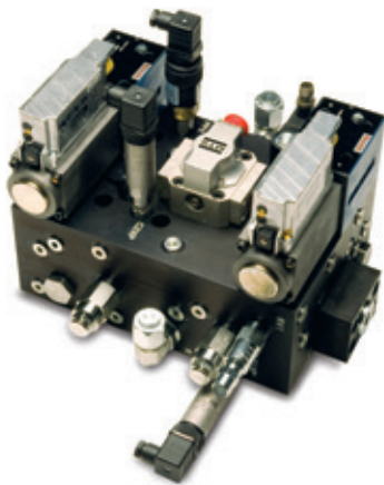
Each MTS Active Load Abort Manifold features a primary and secondary control circuit, as well as a tertiary mechanical fail safe
