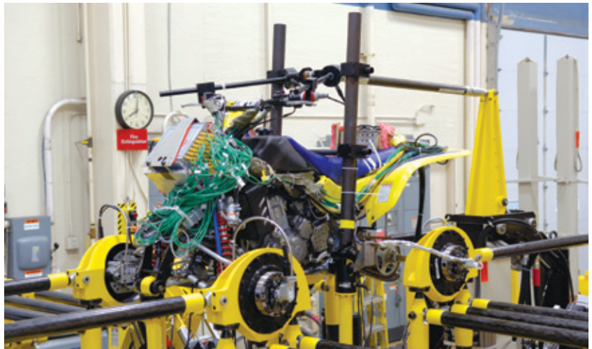
MTS Model 334 Four-Corner Road Simulator
