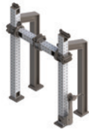
Portal Frame 100 kN dynamic max loads (160 kN static) 300-degree Turning Beam width 65 in, extended max height 84 in
