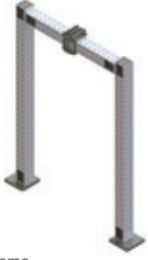
Portal Frame 46.8 kN dynamic max loads (65 kN static) Standard Beam width 59 in, max height 93 in
