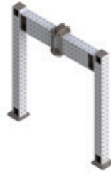
Portal Frame 180 kN dynamic max loads (250 kN static) Cross Beam width 78 in, max height 80 in
