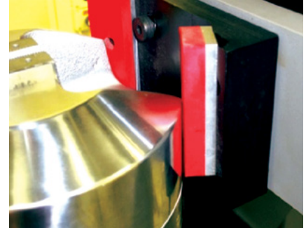
Close-up showing the polymer pads (in this case, red) which restrain the load train components in the event of a compressive specimen failure.
